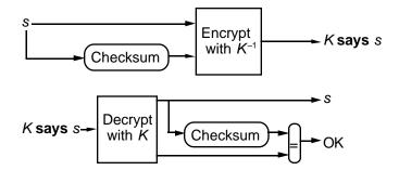
Fig. 3. Using encryption and checksums for integrity.
